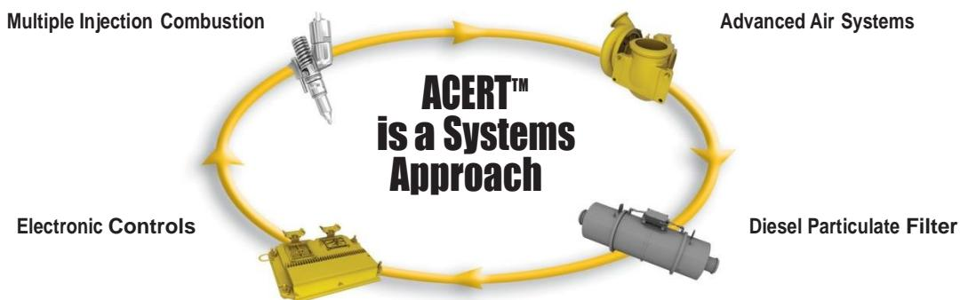
21. The ACERT System uses a Clean Gas Induction ("CGI") process. CGI draws off a small amount of non-combustible gas after it has passed through the engine's Aftertreatment system. The gas is then cooled, blended with more incoming cool, clear air and returned to the combustion chamber. Since the gas is passed through the Diesel Particulate Filter ("DPF"), most contaminants have been removed before the gas re-enters the intake system;
